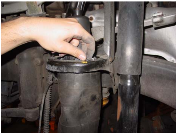
5. Remove the two upper securing clips. ↑
