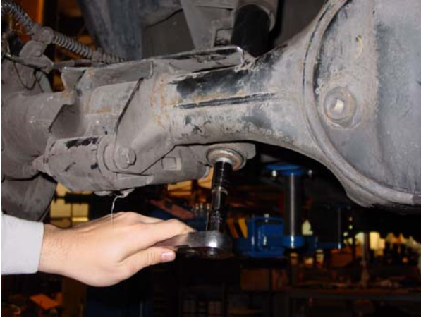
7. Remove retaining nuts from both rear shocks.
