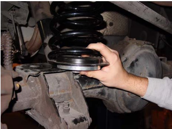
9. Hold the coil spring against the upper mount, while sliding lower spring perch into place. ↑
