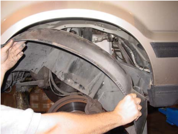
3. Remove plastic wheel arch liner. ↑
