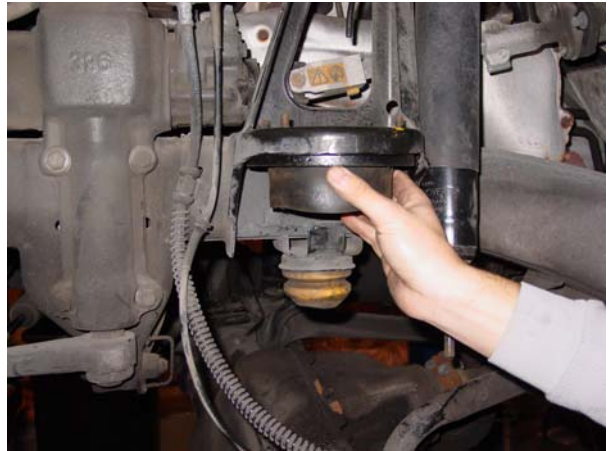
10. Install upper coil spring rubber isolator. ↑
