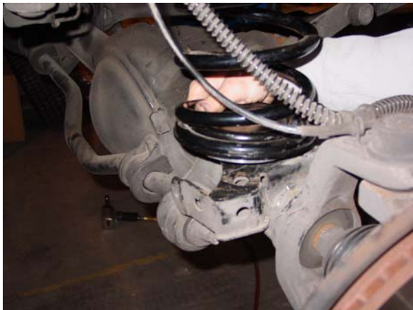
11. Install front coil spring onto the suspension. Hold the coil spring against the upper mount, while sliding lower spring perch into place. ↑
